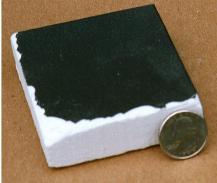
**Figure 2. Sample of space shuttle tile. This piece is from the windward (under) side and coated with a high emissivity coating to enhance radiative losses.**
